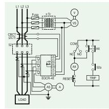
\*For ZCT terminal, it must be used without ground connection.
